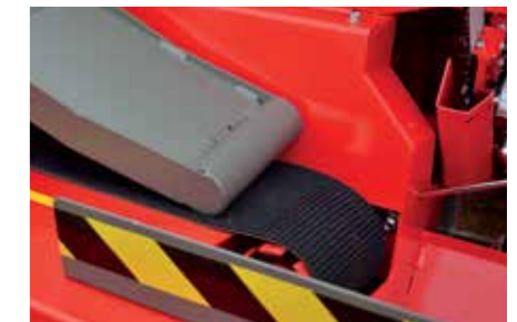
In-feed by means of a conveyor belt in the Standard and Deluxe models (above) and with a spiked roller in the Basic model (below).
