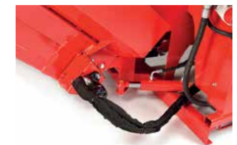
The swivel out-feed conveyor is easy to operate hydraulically.
