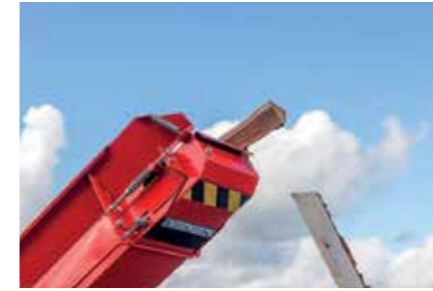
The cleaning out-feed conveyor separates debris, which results in cleaner firewood.
