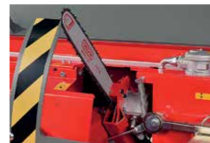
The efficient hydraulic saw operates by keeping the joystick trigger pressed. This minimises the consumption of cutting chain oil.
