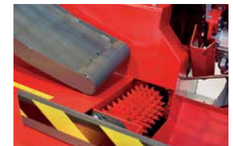
In-feed by means of a conveyor belt in the Standard and Deluxe models (above) and with a spiked roller in the Basic model (below).
