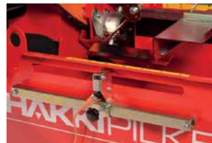
Optical measuring device as standard to ensure desired length of firewood.
