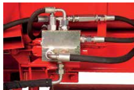
The speed valve accelerates splitting when there is less need for power.
