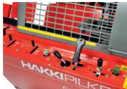
Easy-to-use control panel where in-feed, cutting, and splitting are all controlled with just one joystick.
