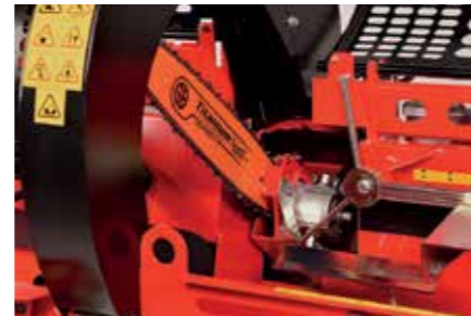
Cutting with a large 20" harvester bar.
