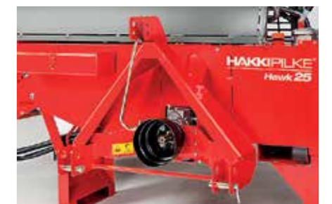
Tractor-powered machines can be transported using the tractor's lifting equipment.
